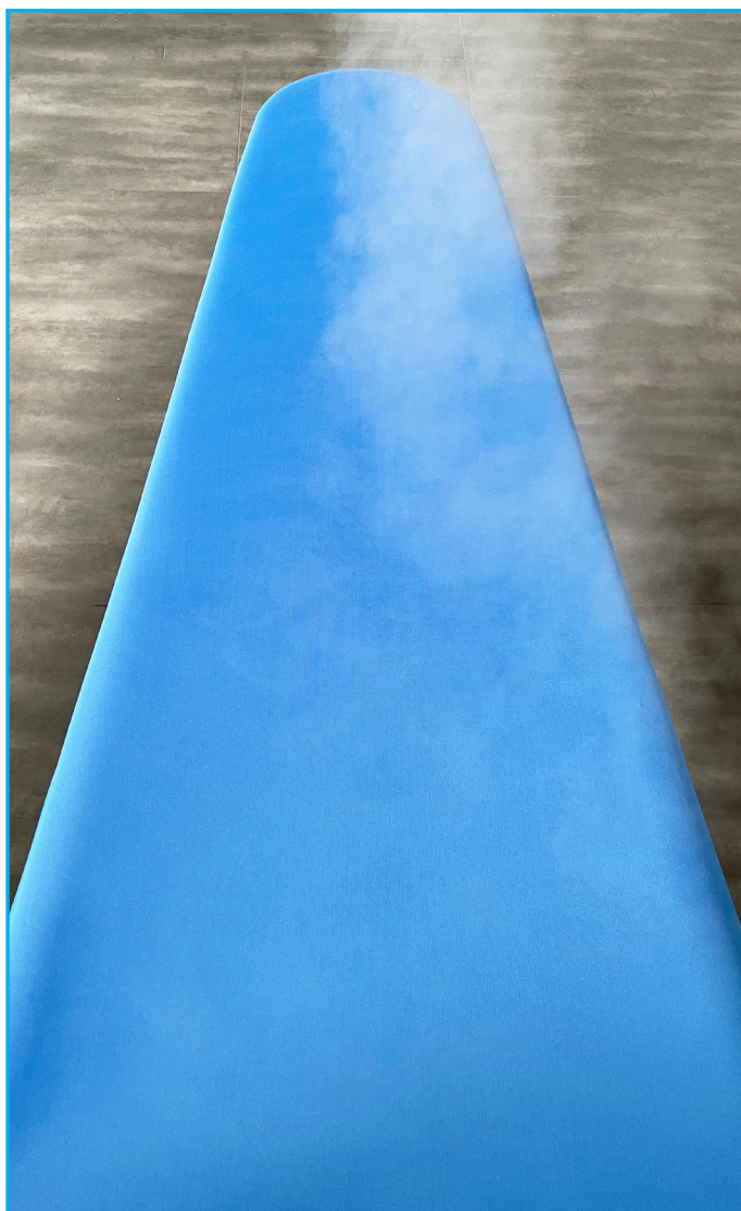
The steam is kept live in a steam chamber under the surface. As the operator steps on the steam pedal, the steam is immediately released in large quantity all over the surface.
