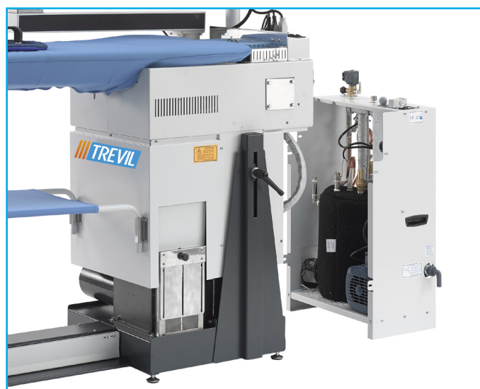
The boiler module includes the 8 lt pressure vessel made of stainless steel, the water pump and the electronic water level control. Two sizes are available: 6kW and 7,5kW. It is removable for easy maintenance.
