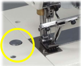
Adjusting stitch length With the push button
