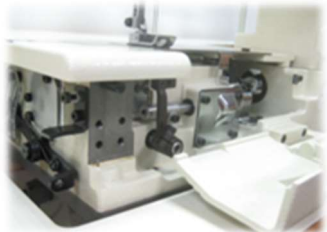
Closed oil circulation system In the feed mechanism
