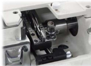
Slide type thread take-up base makes threading and troubleshooting easier
