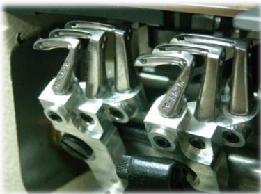
6 loopers pre-installed Split type presser foot
