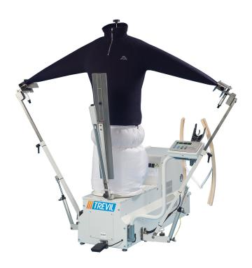
Traditional air / steam form finisher with sleeve tensioning arms. Available with or without boiler.
