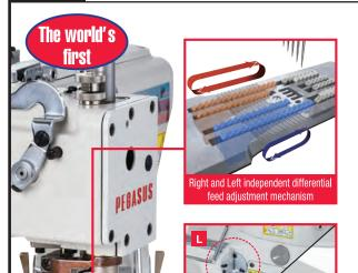
The differential feed ratio can be adjusted separately, in order to respond to operations in which the machine is used to sew right- and left-hand side fabrics that have varying degrees of stretchability, and/or curved lines.
