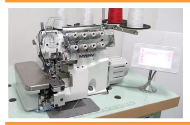
2 needle 4 thread, overlock machine equipped with Ho Hsing automatic back latch device
