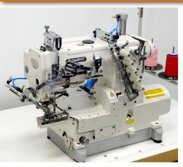
3-needle, top and bottom coverstitch machine with ultra small cylinder bed equipped with pneumatic thread trimmer and direct drive
